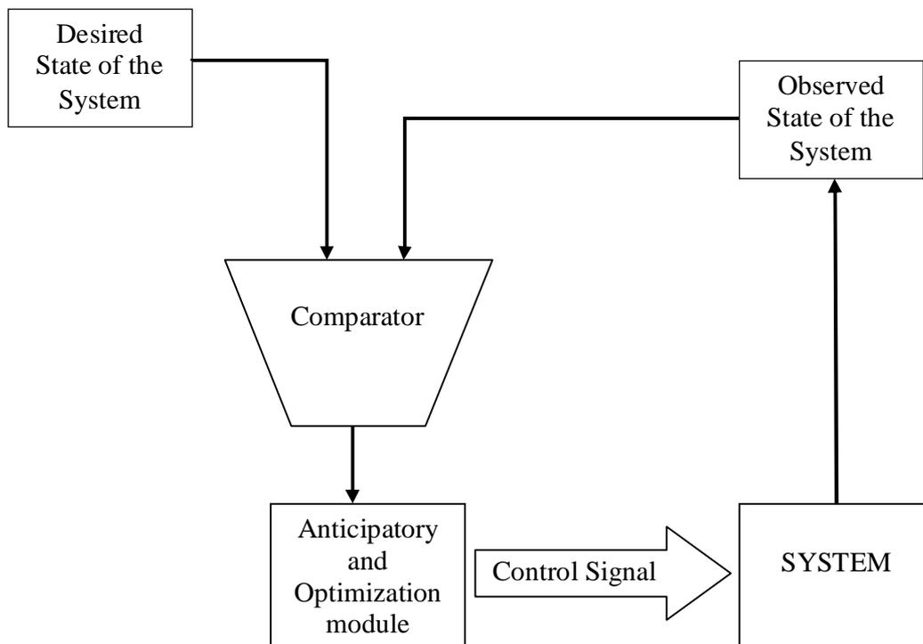
Cybernetics formalizes the above feedback diagram into a finite algorithm: it is essentially a set of concrete rules on what to observe, what to compare to, what to anticipate and how to transmit the control signal to the system.
